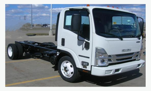
The Isuzu NPR-HD completes our list as a heavy-duty commercial vehicle featuring a 4.8L turbocharged diesel engine paired with a 6-speed automatic transmission. With a power output of up to 215 horsepower and 452 lb-ft of torque, the Isuzu NPR-HD demonstrates impressive capabilities. It has a maximum towing capacity of 12,000 lbs and a payload capacity of 6,825 lbs. Available in standard cab and crew cab configurations, the Isuzu NPR-HD can be upgraded to meet diverse needs.
